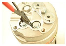
2. Squeeze snap ring that is holding the plug in place.
