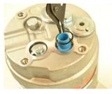
4. Insert snap ring and press around the edges. Ensure that the snap ring seats correctly into the switch port.
